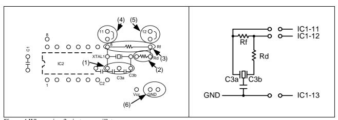
Figure 4 When using 3-pin type oscillator
